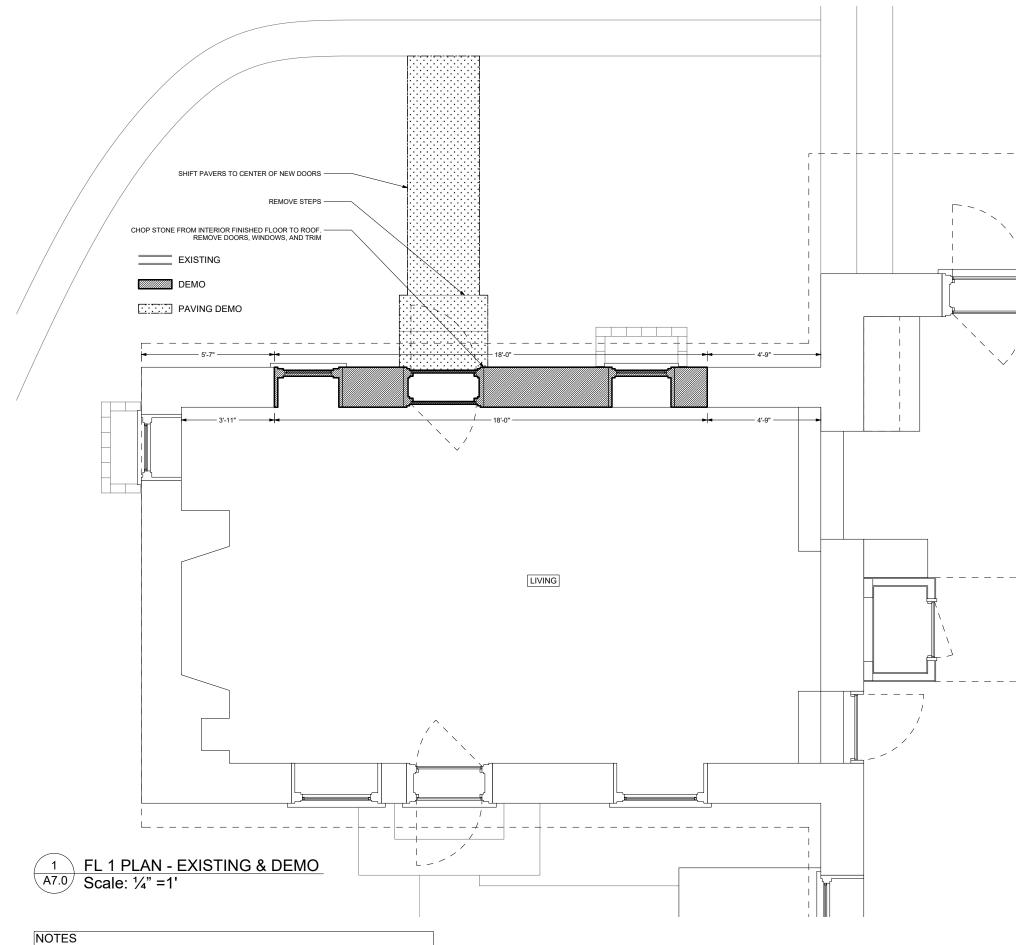
NOTES -PROVIDE SHORING TO SUPPORT ROOF DURING DEMO -RE-USE STONE BLOCKS REMOVED FROM WALL FOR NEW PAVING
